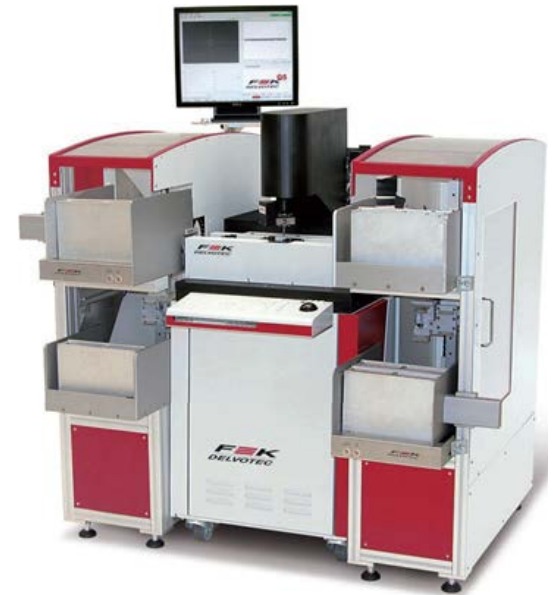
Delvotec 6400 high reliability, high repeatability wire bonding
